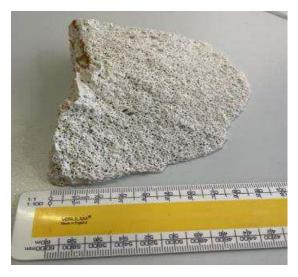
Reinforced Autoclaved Aerated Concrete (RAAC) is a form of concrete with a bubby texture that was commonly used in construction between the 1950s and 1990s. Its aerated texture means it is much lighter than typical reinforced concrete, but not as strong. It was predominantly used in a wide range of buildings as precast panels or planks in roofs (generally flat roofs, although sometimes pitched) and occasionally in floors and walls.
